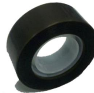
TOOL-017 30' Teflon tape roll (used for hard cards to reduce scratching)
